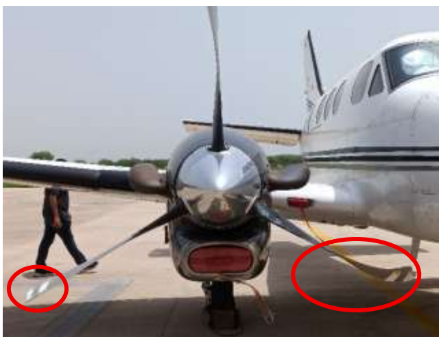
FIG 2: Damage to RH Propeller
