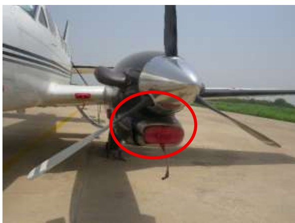
FIG 3: Damage to LH engine intake and propeller
